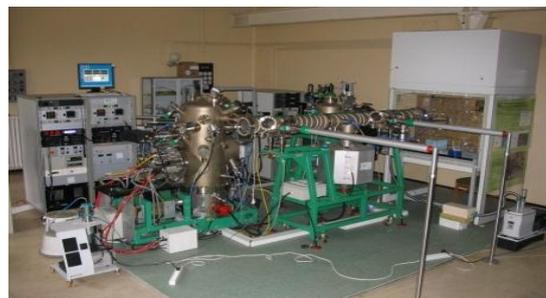
The MECA-2000 molecular-beam epitaxy facility for preparing metallic thin-film samples under ultrahigh-vacuum conditions
