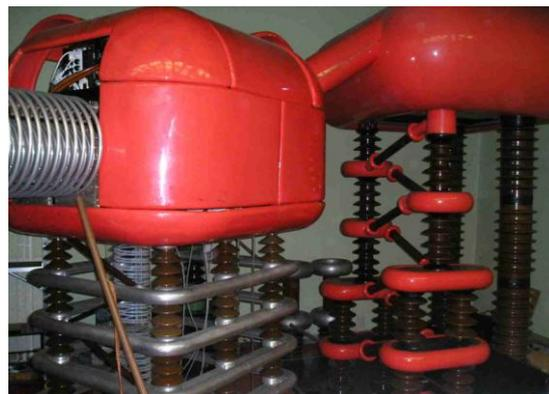
The NIK heavy-ion implanter of 450 kV terminal voltage
