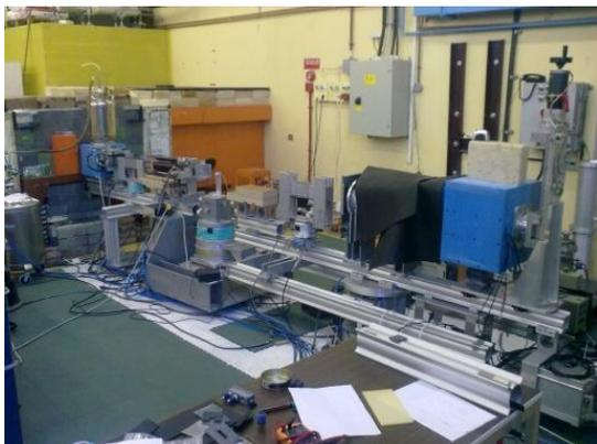
The GINA polarised neutron reflectometer in operation at the neutron guide hall of the Budapest Neutron Center (BNC)
